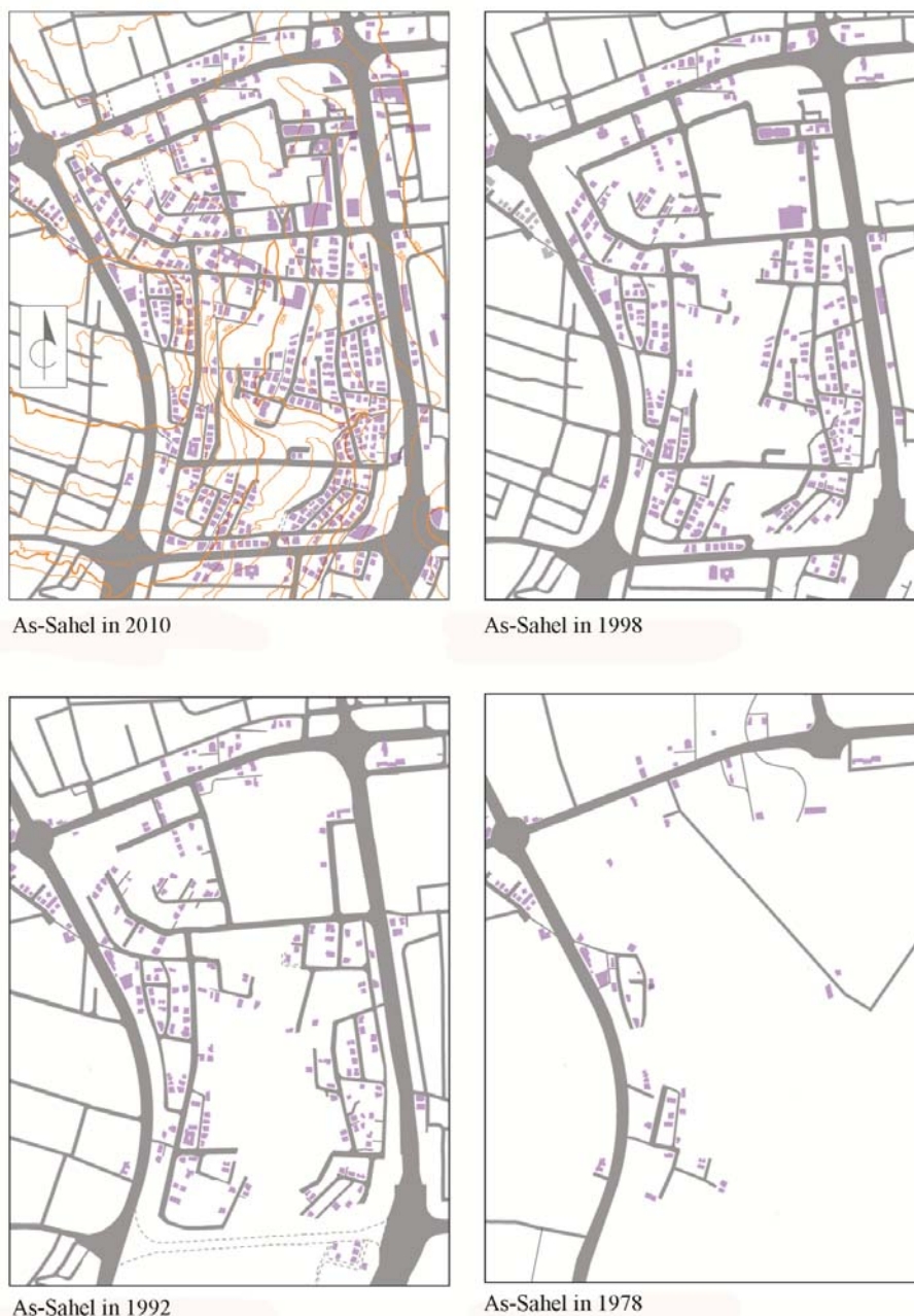
Figure 14. Urbanization process in as-Sahel at five different stages - showing the effect of population influxes post 1992, and post 2006. (Source: Source: Author, based on field work, aerial photos of 1992, 1978 from the Royal Geographic Centre, and Amman 2005 GIS)
